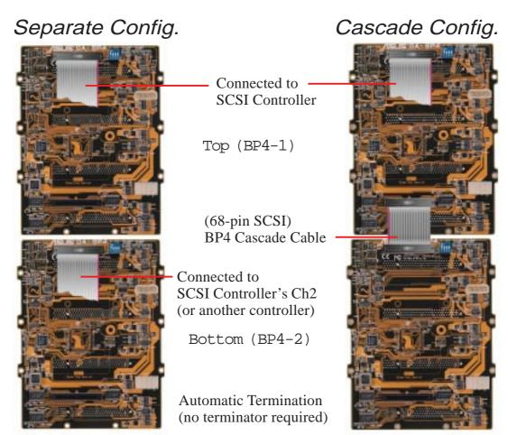
When using a cascade configuration, the top SCSI backplane board is referred to as BP4-1 and the bottom SCSI backplane board is referred to as BP4-2, but there are no physical differences. The SCSI hard drives connected on the top SCSI backplane board may select from two sets of SCSI IDs. The SCSI hard drives connected on the bottom SCSI backplane board may only have one set of SCSI IDs.
